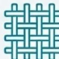
**The Reinforcement:** Fiberglass mesh (60-80 g/m<sup>2</sup>) for structural integrity on complex surfaces
