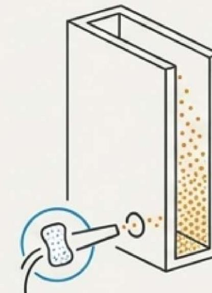
Blowing the granulated cork into the cavity, starting from the lowest point and working upwards. Use of a sponge plug minimizes dust.
